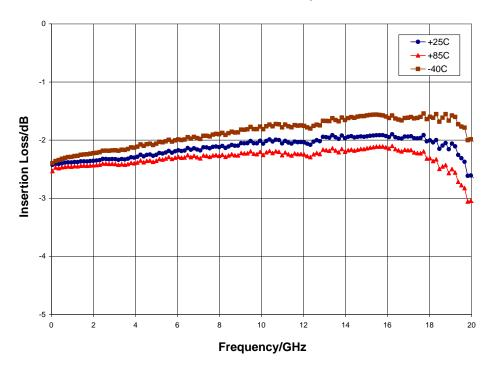
Insertion Loss vs. Temperature
